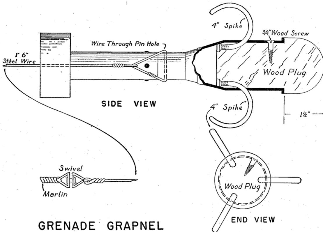
**Firing Procedure and Range** The normal firing procedure for the AT Grenade M9A1 is followed. Extra care is taken that the trailing wire and cord are free of the grenade launcher and rifle, and that the trailing cord is carefully coiled on the ground, preferably to the right of the weapon. With the rifle at a 45° angle, the grapnel will attain a range of 75 to 100 yards.
