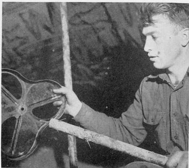
Cloverleaf prevents tearing camouflage netting.
